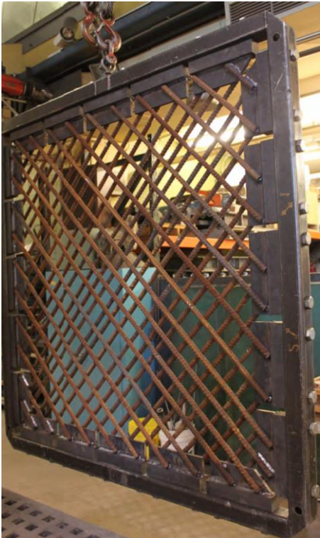
Figure 1. Welded Reinforcement Cage (Half Specimen)
