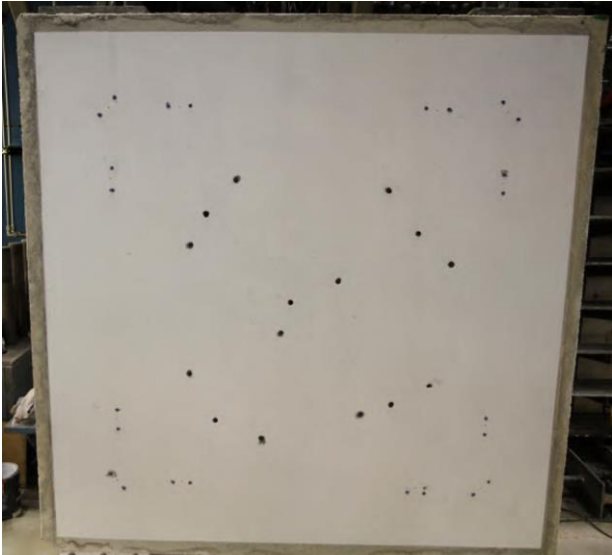
Figure 4. Completed Shell Specimen
