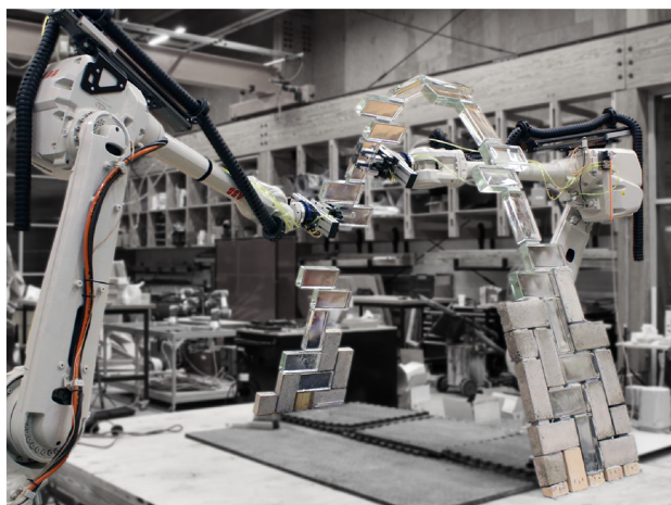
(b) Approaching the end support of the arch. Additional bricks close to the base provide lateral support.
