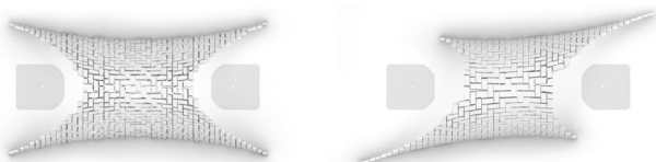
Fig. 4 Original geometry based on line symmetry (left) and adjusted geometry based on rotational symmetry (right)
