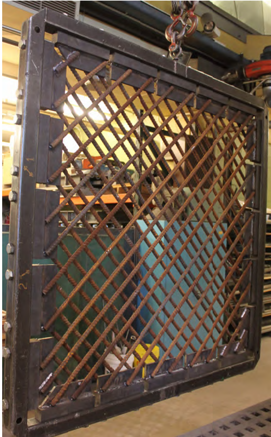
Figure 3.3: Welded Reinforcement Cage
